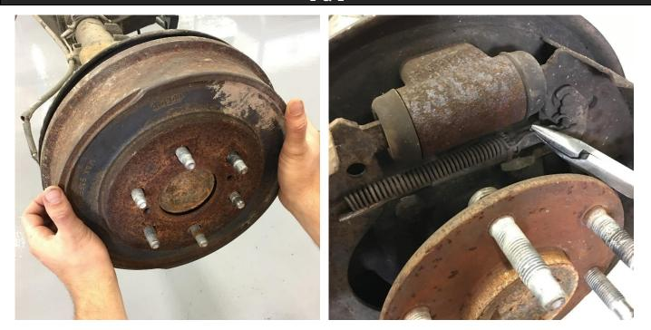
This installation refers to the **passenger side** of the axle. All steps are to be repeated on the driver side. Start by removing the factory drum. It may be necessary use a lubricant around the axle register to do this. Once the drum is removed, remove the first brake shoe retaining springs as shown.
