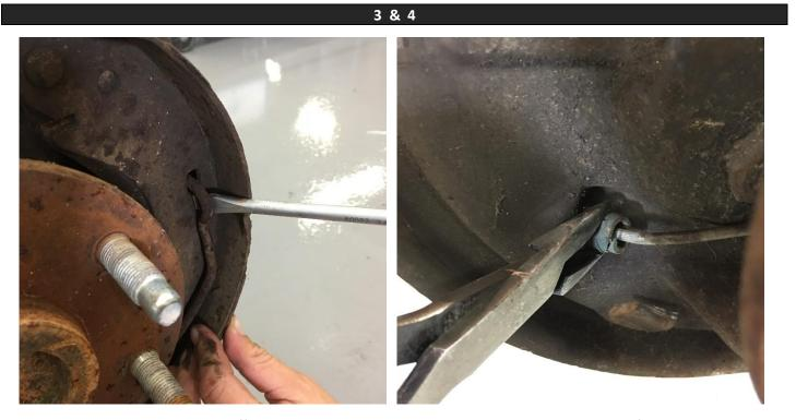
Remove the brake shoes by prying off the retainers on each side. The cable can then be removed from the backing plate by depressing its perimeter springs and pulling it through.
